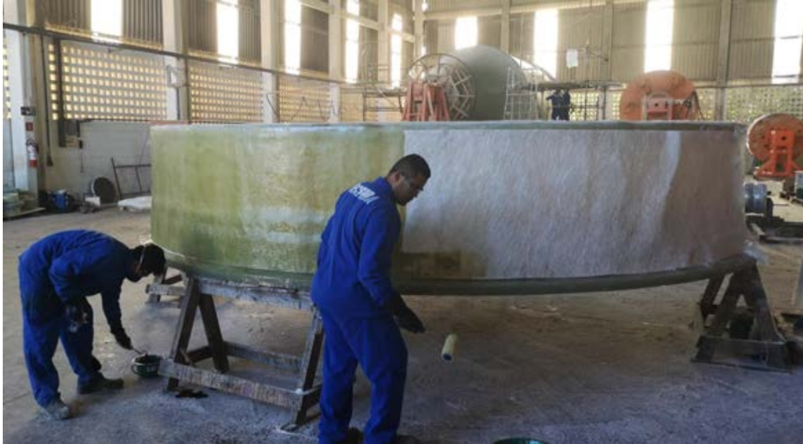
Figure 4: Eliminating air bubbles.
