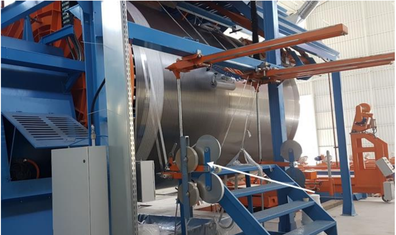
Figure 12: Mylar unwinder with Mylar detection sensor, and veil unwinder
