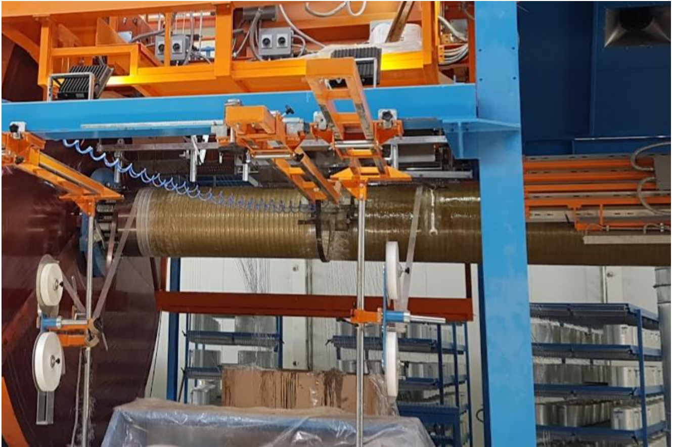
Figure 17: Compaction roller, finishing roller, surface veil unwinder
