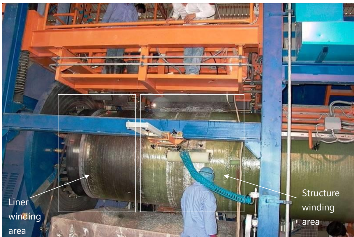
Figure 11: EFW winding area (with marked liner and structure winding areas)
