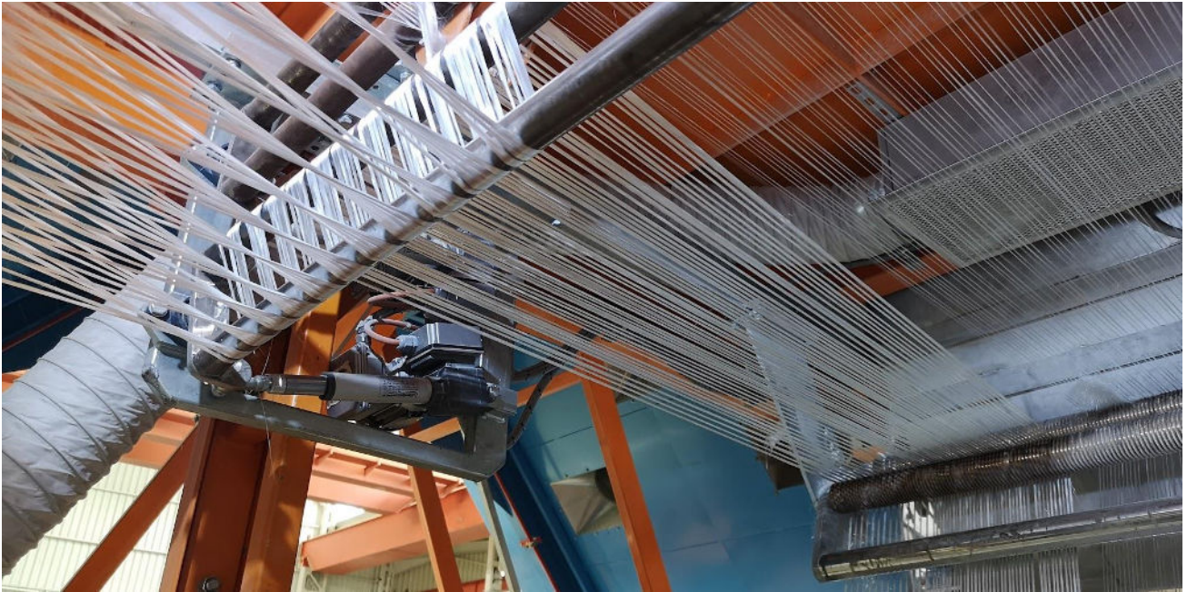
Figure 13: Hoop roving guide, hoop tensioner and combs
