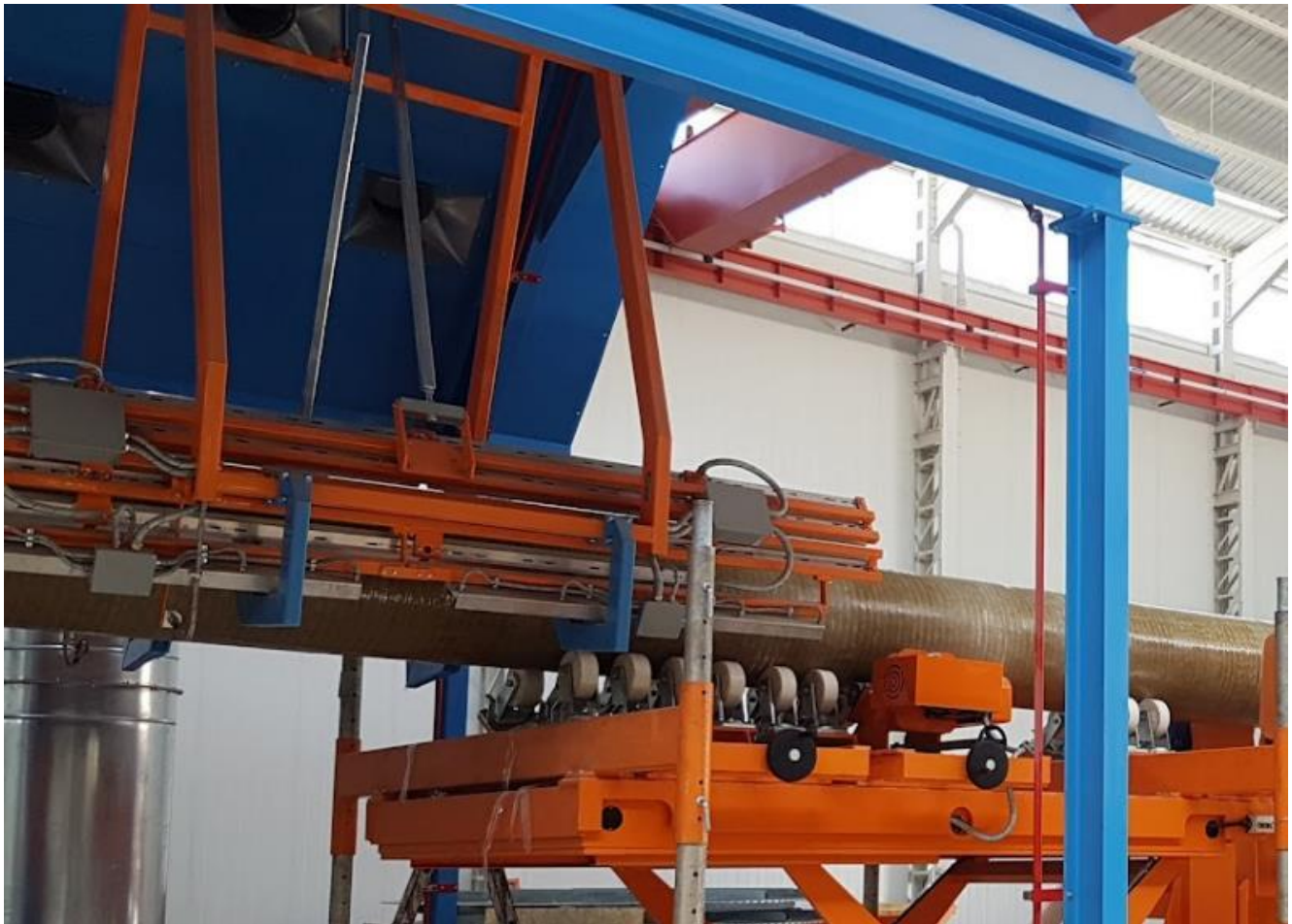
Figure 18: Curing station with IR lamps
