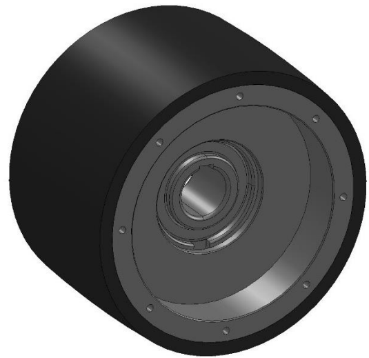
Figure 17: Removed wheel side cover with shaft and bearing housing
