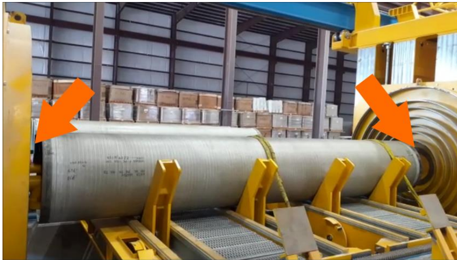
Figure 30: Pipe during extraction from fix head
