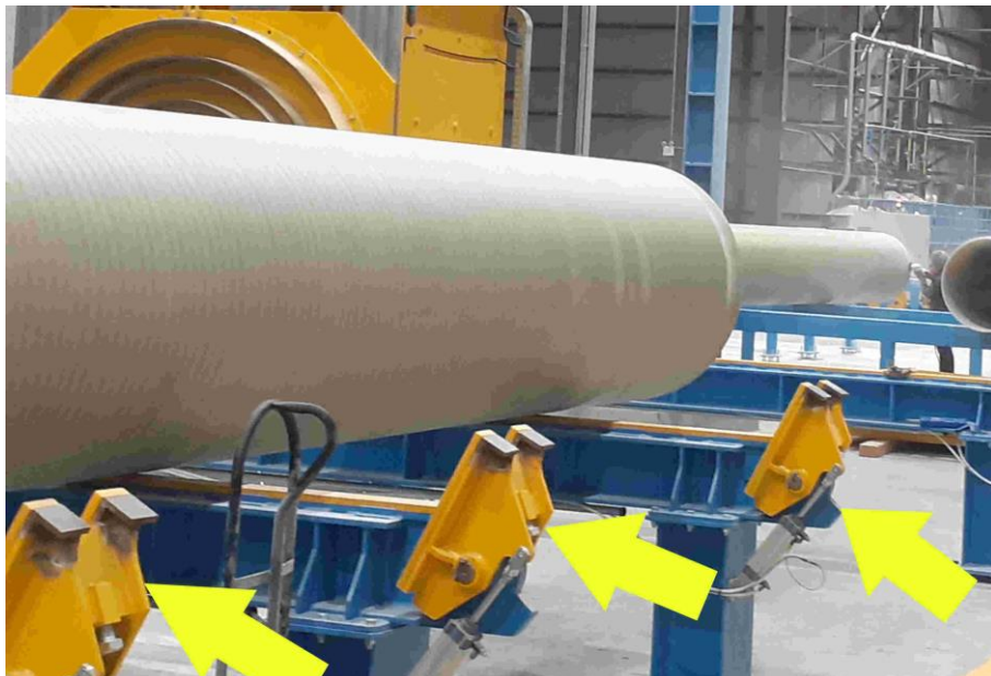
Figure 25: Outer stoppers swivel upwards
