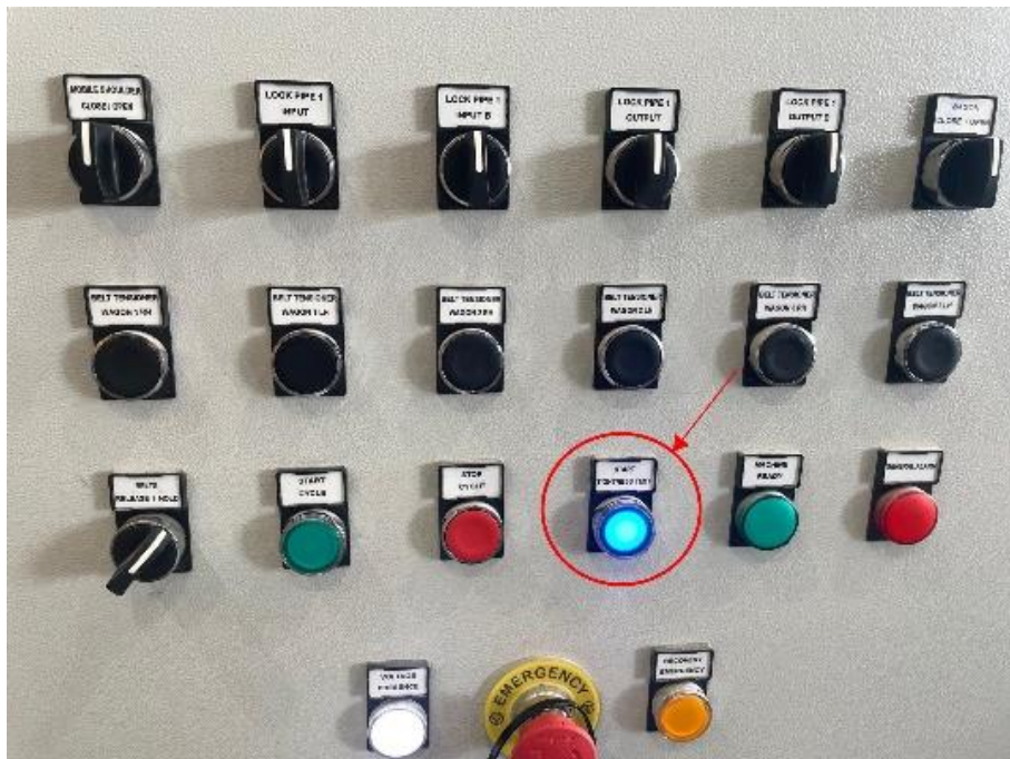
If there are no leakages, press the flashing blue button again.
