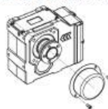
Fig. 10: Protection cap for shrink disc hollow shaft
